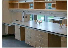
**Adjustability** - Sigma Fusion™ can accommodate a number of workstations at varying heights in a single work area. Height adjustable work surfaces vertically adjust in 1" increments from 30" to 36"; allowing to ergonomically design work stations to accommodate the requirements of individual users and the different procedures and equipment.
