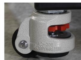
**Effortless Mobility** - Swivel casters have an adjustment knob that lowers the pad and raises the wheel off the ground to prevent rolling. Perfect for applications where work demands stability and a level work surface.
